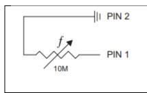
In simple terms, the Force Sensor Touch is a layered electrical membrane based on a specialty resistive ink on one layer that varies in resistance value as it is being pushed.
